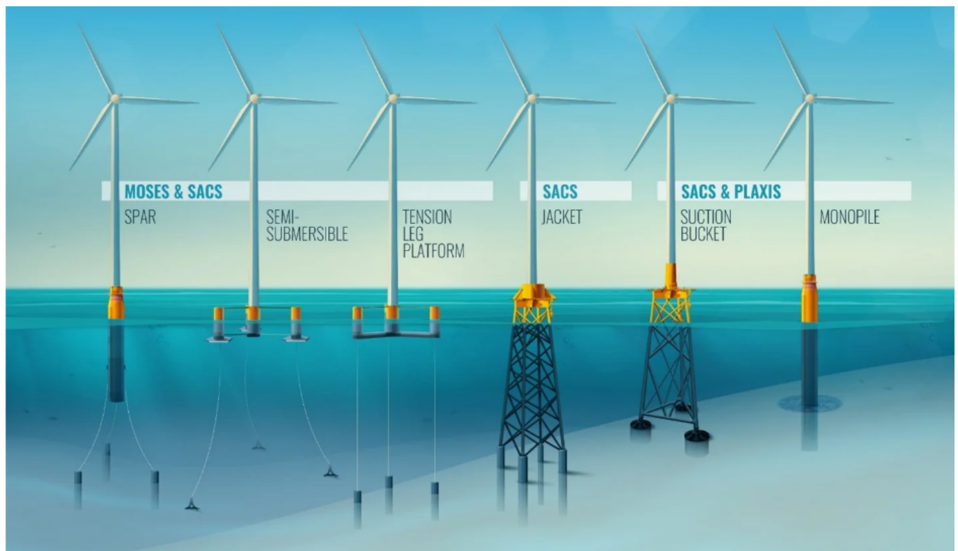
Figure 11: Floating platforms of shore turbine
