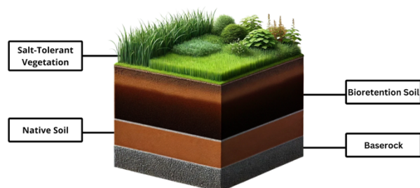
Figure 4.1.10 Cross-Section of the Saltwater Intrusion Bioretention System.
