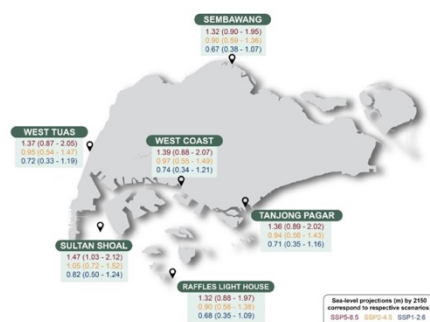
Figure 1.4.2 Projected relative sea-level rise in Singapore at six tide gauges by 2150. The tide gauge that is nearest to the Pandan Waterway will be the West Coast tide gauge 12 .
