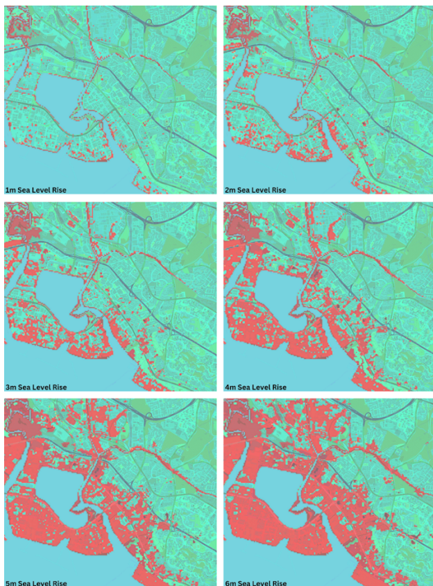
Figure 2.3.2 Effect on sea level rise (1-6 m) on the low-lying land by the Pandan waterway. Red Indicates Submerged Area. Elevation data was sourced from OpenTopography and processed with QGIS for spatial analysis and visualisation.
