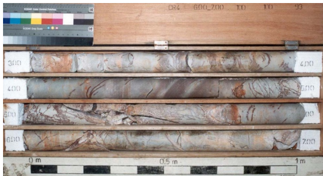
Figure 2.3.1 Sandstone Layers from Pandan Drainage Catchment Borehole 34 .
